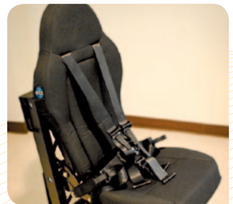
GSS's new military seat with foam & comfort development executed in ESI's PAM-COMFORT
