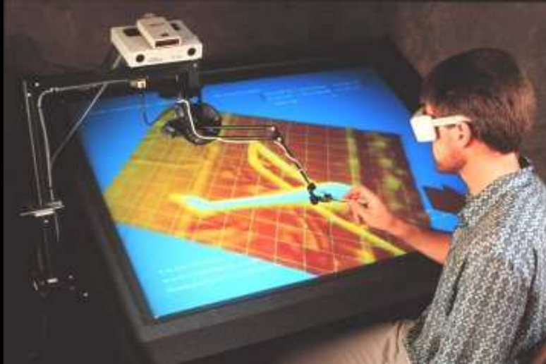
feeling carbon nanotubes with an Atomic Force Microscope
