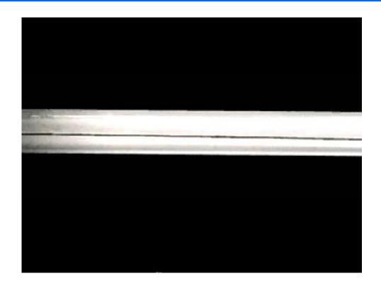
In this experiment water flows through a clear pipe with increasing speed. Dye is injected through a small diameter tube at the left portion of the screen. Initially, at low speed (Re <2100) the flow is laminar and the dye stream is stationary. As the speed (Re) increases, the transitional regime occurs and the dye stream becomes wavy (unsteady, oscillatory laminar flow). At still higher speeds (Re>4000) the flow becomes turbulent and the dye stream is dispersed randomly throughout the flow.
