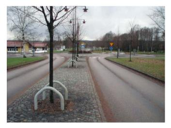
**Fig. 5.** Narrow lanes for cars and busses, vulnerable road users on parallel roads, roundabouts as crossings in city of Borlänge, Sweden. This type of design reduces fatalities by 80–90%.
