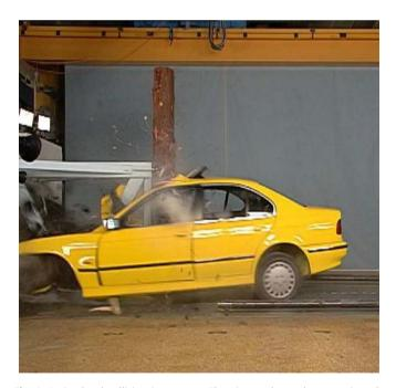
Fig. 4. A simulated collision into a tree. The picture shows the approximately position of the tree after a 70 km/h crash.
