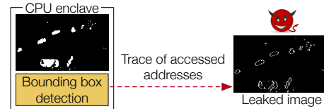
Figure 2: Attacker obtains all the frame’s objects (right) using access pattern leakage in the bounding box detection module.
