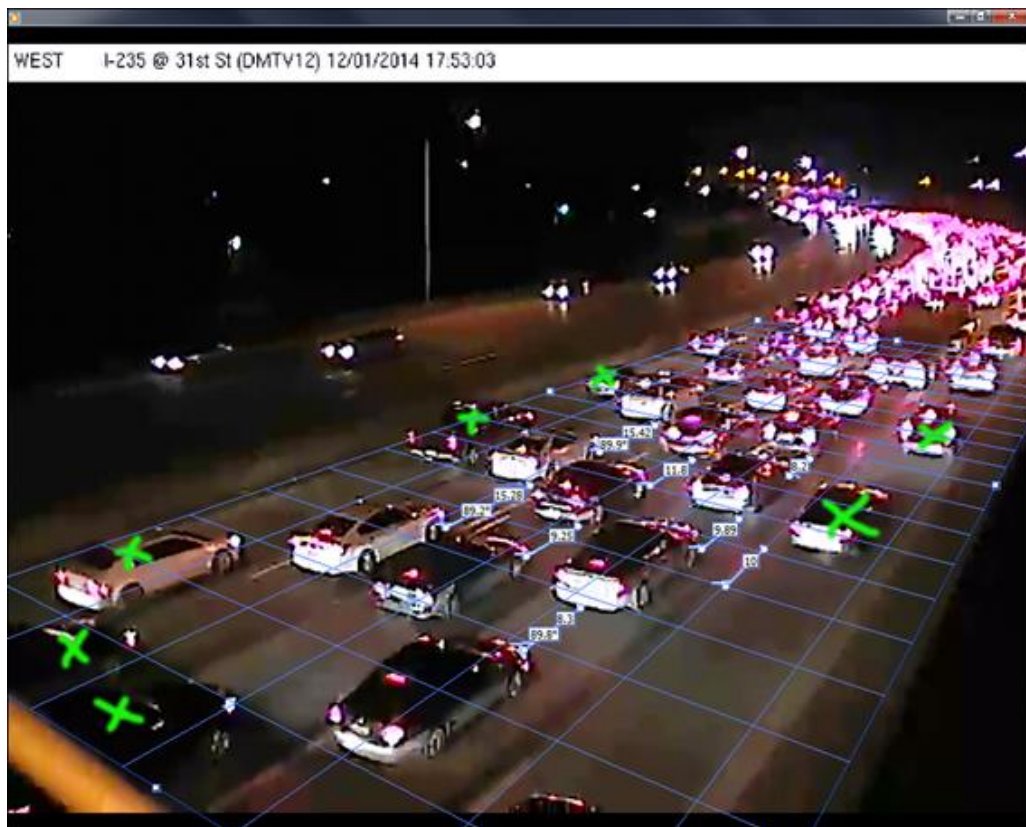
Figure 15. Example of an image processed for standstill distance measurements
