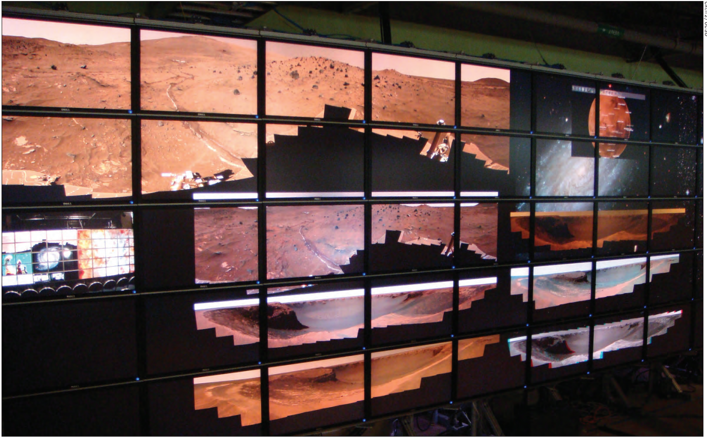
Figure 3. The 70-tile, 286-megapixel Highly Interactive Parallelized Display Space (HIPerSpace) OptIPortal, developed by the Calit2 VisGroup, displays ultra-high-resolution imagery from the Mars Exploration Rover Mission in different wavelengths, notably, McMurdo, Cape Verde, and Duck Bay.
