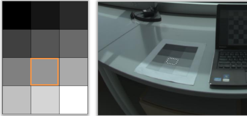
Figure 41 Test Case: Image Luminance Calibration
