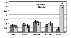
Wear testing of polished materials against natural human tooth structure was performed. The volume loss of the material and the natural tooth enamel was measured. The enamel loss of Vita Mark II, Procad and Mz100 were all statistically equivalent. The loss of material itself was higher with Mz100.
