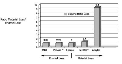
If the enamel versus enamel test is normalized to a value of one, then we may rank the test materials relative to enamel versus enamel wear loss. Values close to one indicate wear behavior similar to enamel versus enamel. Values higher than one indicate loss of the material itself. The data indicates that Mark II is a wearkind material, which does not deteriorate during tooth contact.
