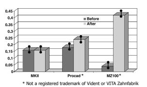
The surface roughness of materials was measured before and after the wear test. There was no change in surface roughness of the Mark II. Procad became about 30% rougher and Mz100, although initially the smoothest became 700% rougher. As surfaces become rougher they may become dull and also may tend to accumulate more plaque than smooth surfaces.
