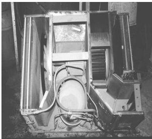
Figure 54. A window air-conditioning unit with cover removed (the compressor is at bottom, condenser coil on the left and evaporator on the right).
