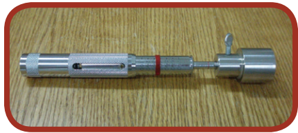
Figure 17: A pocket penetrometer can be used to determine CLSM strength prior to backfill
