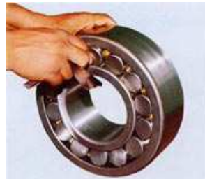
Fig: 13.0 Insert the feeler gauge between top rollers and outer race to check radial clearance.
