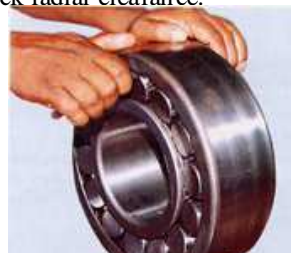
Fig: 14.0 Checking radial clearance over both rows of rollers simultaneously
