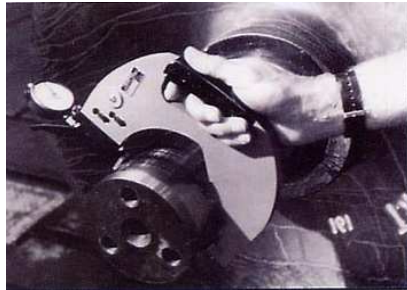
Fig: 9.0 Use of dial snap gauge for checking journal diameter
