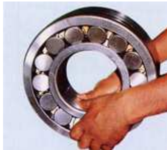
Fig: 11.0 Oscillate inner ring two or three times, pressing down firmly
