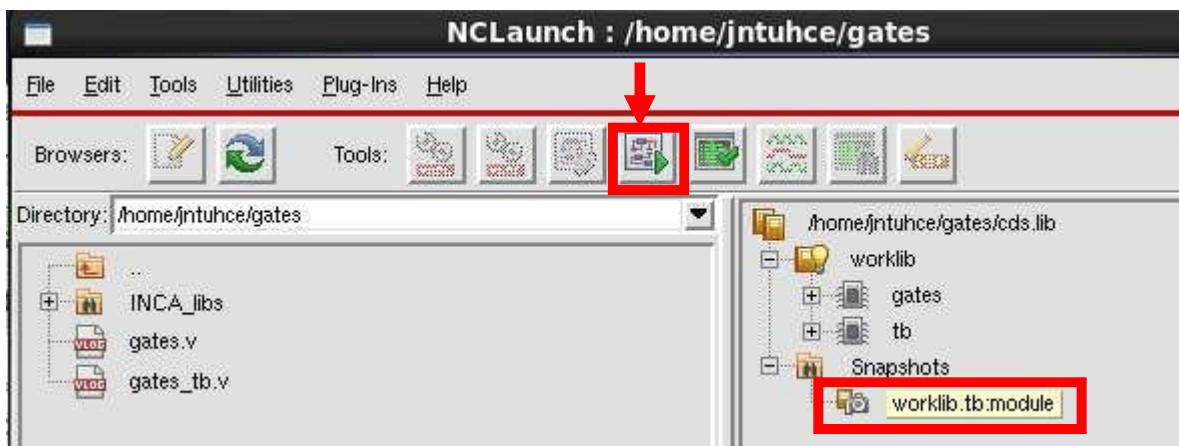
Select simulator to simulate the design. After simulation you will get the two windows like below image.
