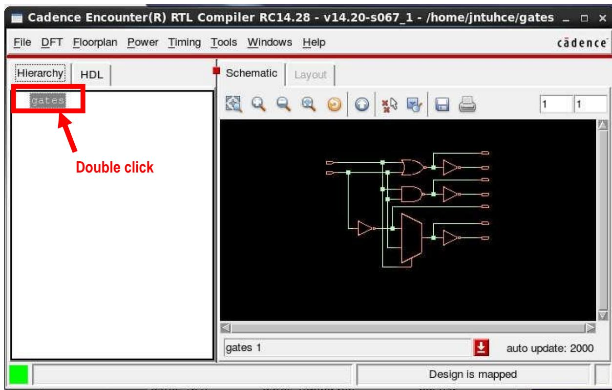
This will show the RTL schematic of the netlist generated.
