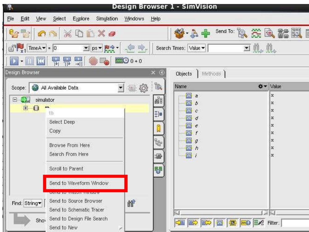
select the testbench for the gates and Rightclick it. Select the send to waveform window or select the waveform icon
