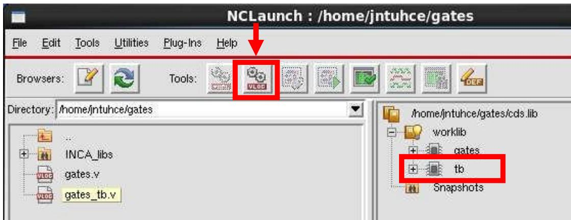
Select the testbench and compile it. It will come under worklib. Under Worklib you can see the module and testbench. Next is to elaborate the design.
