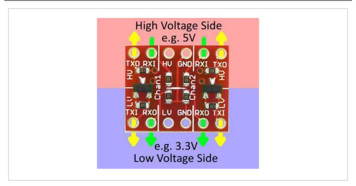
To send a signal from the low-voltage side to the high-voltage side (e.g. from 3.3 V to 5 V), the signal must be input at TXI. It will pass through the converter and come out as a higher voltage on the TXO (transmit output) pin.
