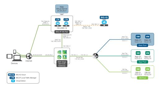
Connecting the BIG-IP VE to NSX Edge and Internet using two network interfaces.
