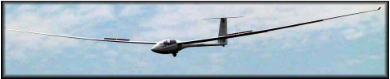
Tony Elliot brought two 10.3 meter span models, one being an ETA, a scratchbuilt model that uses a much modified Rosenthal ASH-25 fuselage. AUW of 45 lb. and aspect ratio of 53:1, each wing panel is made up of 3 sections.
