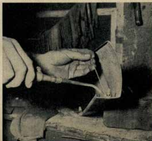
16 Now weld studs onto each of straight bar pieces so that headlight shells can be attached properly to straight grille bars. 125
