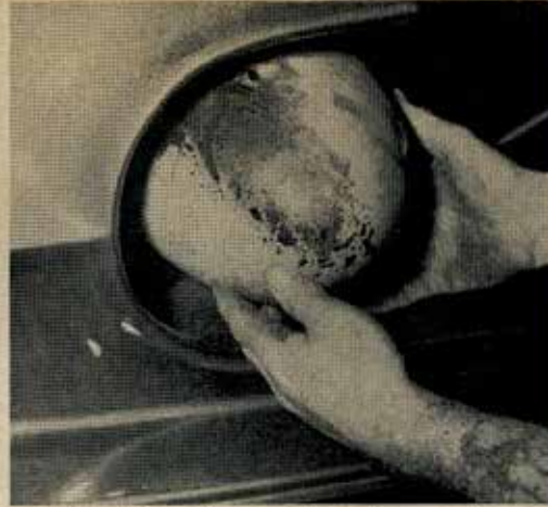
6 Allowing at least an inch clearance between grille shell and newly shaped oval, align and reshape the shell as required.
