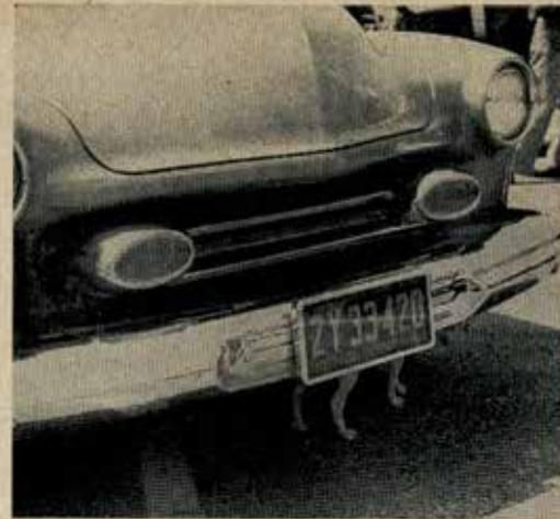
A '55 Oldsmobile grille bar floats inside '51 Merc shell. Inside bar are right and left handmade lucite directional lights.
