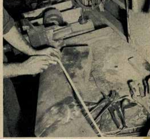
8 Transfer this measurement, after checking carefully to be sure it's correct, onto the accessory grille bar to be used on car.
