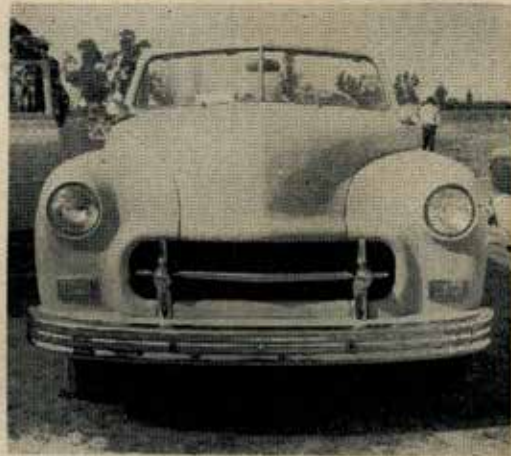
Floating grille on this early-model Dodge is made from straight bar with two bumper uprights vertically matched to shell.
