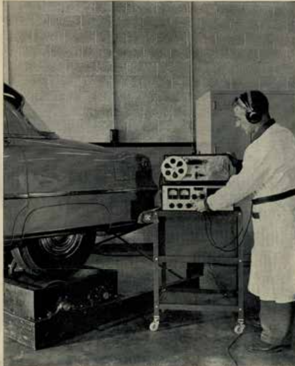
Car speeds up to 70 miles an hour can be duplicated in this sound laboratory. Checking on noise deadeners and sound absorbers with tape recorder is Charles Simler, of the Fisher staff at the GM Proving Ground. Microphones are placed inside automobile.
