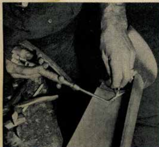
15 Weld bracket onto each of straight grille bars so that holes align with the drilled holes in both of the headlight shells.
