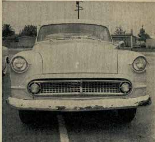
Floating grille consists of two right and left '55 grille end pieces formed to fit the '53 Chevrolet parking light housings.
