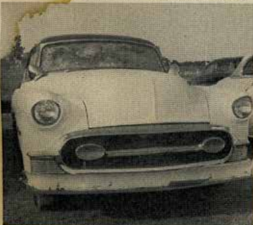
Inside of this grille on '53 Chevy, '54 Oldsmobile bumper bar is used. It is attached from rear of the inner pan assembly.
