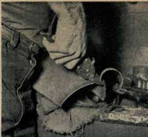
11 The fit, in this case, was not quite satisfactory, so here the customizer is using metal shears to trim off the excess metal.
