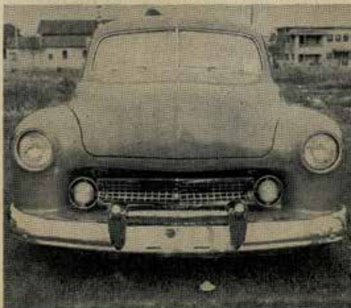
A '55 Ford grille has been adapted to fit this '50 Mercury; '53 Chevy parking light housings float, using inner-type brackets. 127
