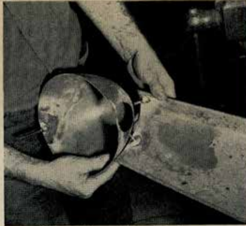
18 With each straight grille bar on a bench, attach each of headlight shells to straight bar, using studs already installed.
