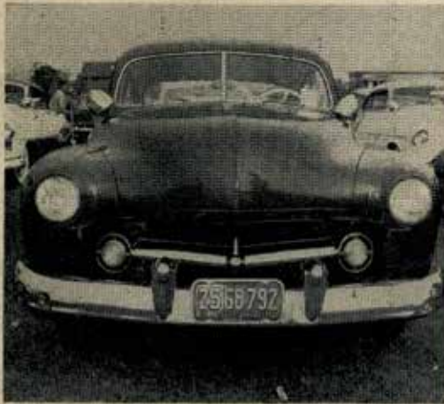
A '53 Chevy grille bar is cut down and re-V'd to match the grille shell opening. It uses vertical grille tooth at the center.
