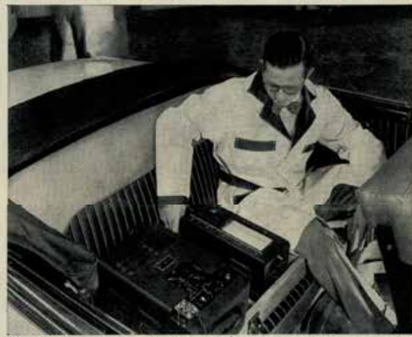
Ultra-sensitive strain gage enables Fisher Body engineers to check within a millioth of an inch the amount that any particular piece of metal stretches under driving conditions. Richard Mitchell, of the Fisher staff at GM Proving Ground, is testing body mount.
