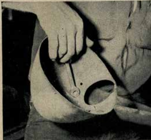
19 Secure the headlight shell installation on the straight bars by tightening the nuts slipped inside shell onto each of the studs.
