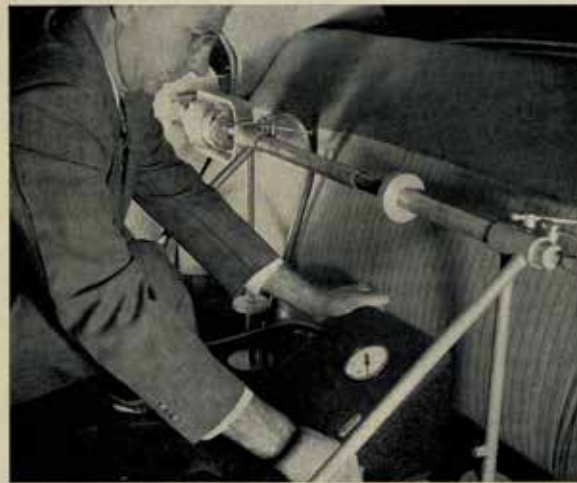
Pressures of up to 400 pounds per square inch can be put on doors of Fisher bodies with this brace which tests holding power of door locks and latches. Pneumatic device is set up at GM Proving Ground, then car is driven over famous Belgian block road.
