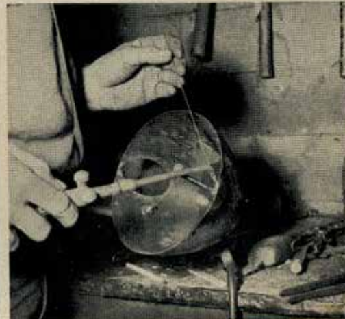
20 Now braze studs onto light shell for attaching floating bar and light shell assembly to each of the fender inner panels.
