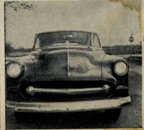
22 Here is finished product: a custom floating grille that has been installed in a custom-molded '53 Chevrolet grille shell.
