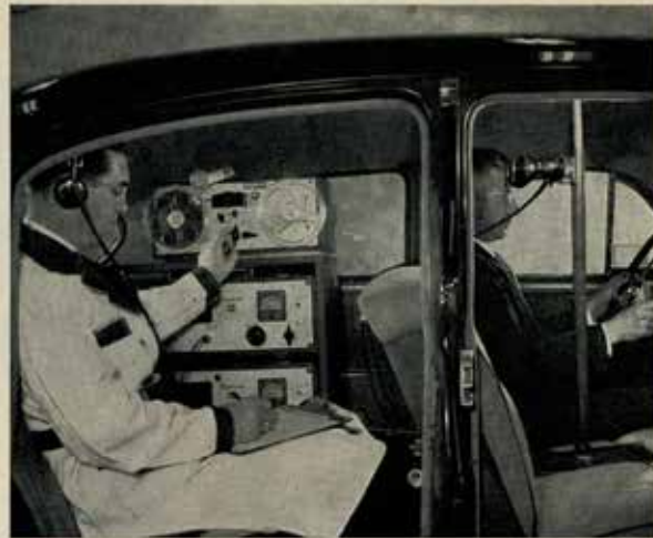
Double microphones do for this tape recorder what stereo lenses do for a camera—give greater depth. Marden Locey, left, GM Proving Ground, and Charles Simler, Fisher Body, make recordings of body noises to study effects of different types of insulation.
