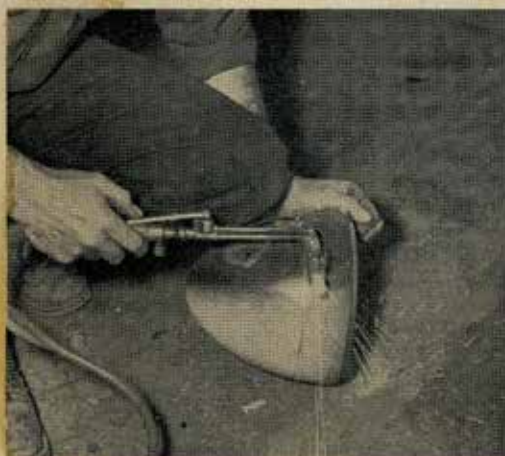
3 Using cutting torch, apply heat along marked line on headlight shell to cut all excess metal as determined by measurements.
