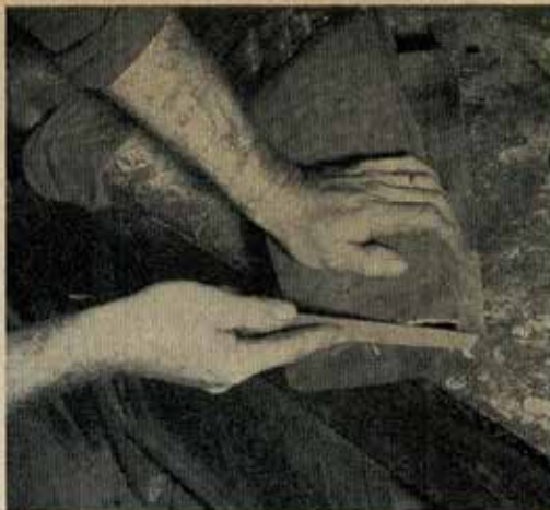
12 Using a half-round machine file, cut sections are now thoroughly cleaned and filed to make as close a fit as possible.
