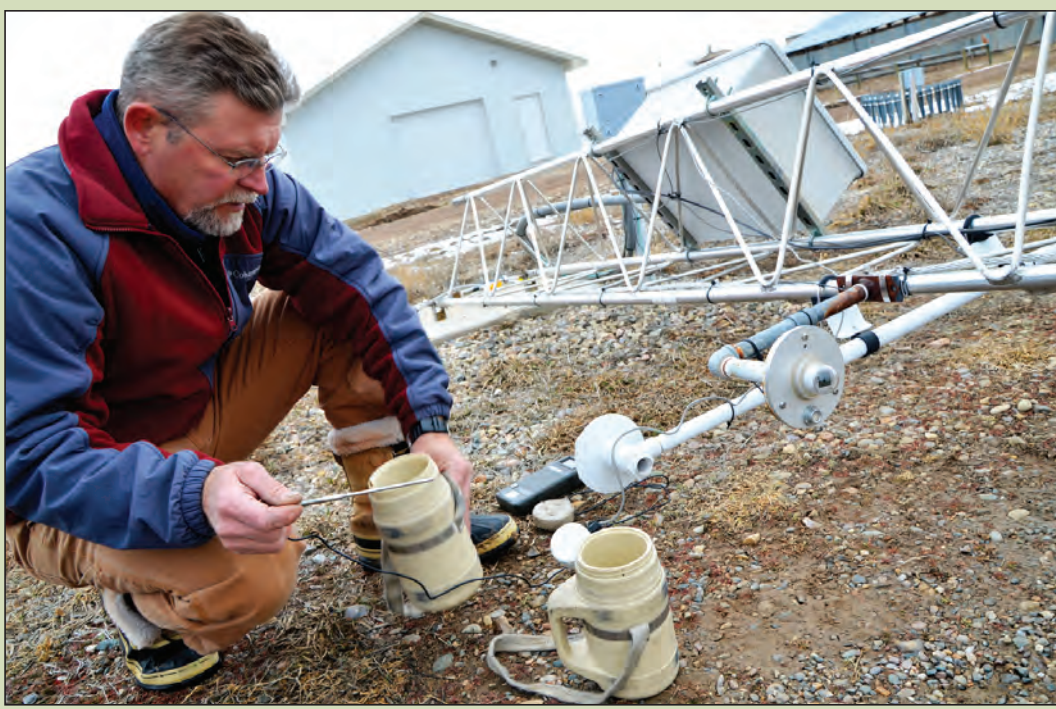
Martin Valvur of Air Resource Specialists Inc. of Fort Collins, Colo., sets up a field test to compare the accuracy of the air monitoring equipment operated by the Southern Ute Air Quality Program on Tuesday, Feb. 14 at the Ute 1 site in Ignacio. It's critical that the AQP's instrumentation is within EPA parameters prior to submitting data to the EPA. Temperature sensors, one of many meteorological parameters measured at the Ute 1 station, are placed in an ice bath and heated water bath to measure the accuracy of the temperature sensor across a range representative of ambient conditions. A solar radiation sensor measures light intensity associated with direct sunlight. All factors have a direct influence on the immediate air quality. Calibrations are typically performed at the air monitoring station every three months.
