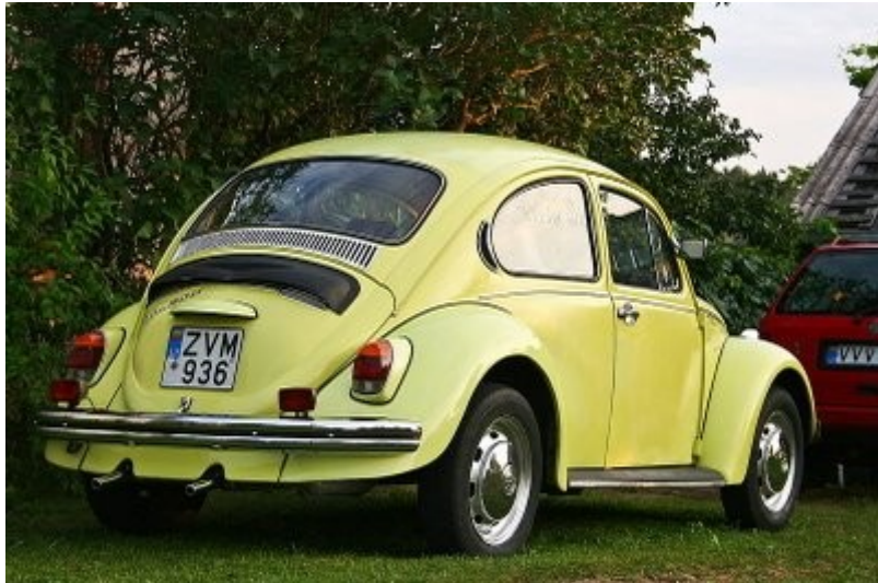
VW 1300 (1972) with an aftermarket rain shield over the engine hatch air vents.
