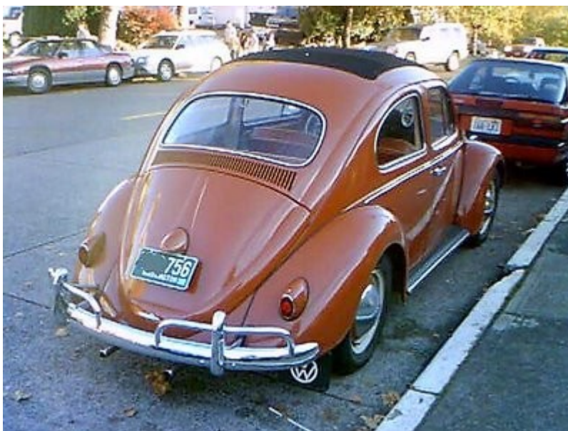
1961 VW Beetle rear view. Narrow licence plate light cover, wide rear window, simple tail lens, bumper over-ride guards.
