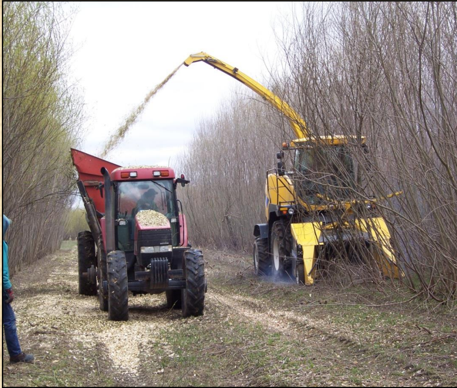
New CNH Short-Rotation Coppice header being tested in western NY in early 2009
