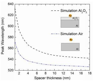
Figure 6. Gold nanoparticle scattering peak wavelength obtained using numerical simulations with either an  $Al_2O_3$  film or an air gap as a spacer layer between the nanoparticle and the Al substrate.
