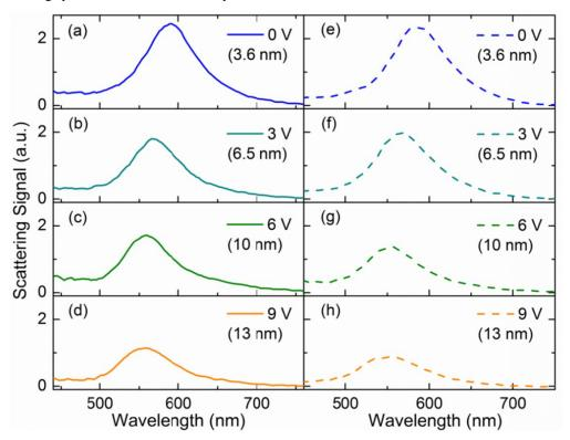
Figure 2. Single particle scattering spectra from two gold nanoparticles after four anodization steps (a)-(d) (solid lines) and (e)-(h) (dashed lines). The corresponding  $Al_2O_3$  thickness after each anodization step is shown in parentheses.
