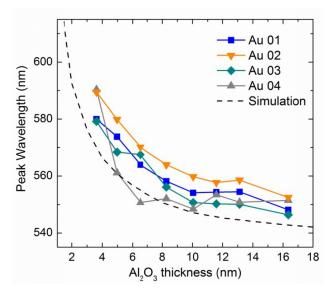
Figure 4. Fitted peak scattering wavelength of four individual gold nanoparticles as a function of Al<sub>2</sub>O<sub>3</sub> thickness, as well as the corresponding simulated peak position (dashed line).
