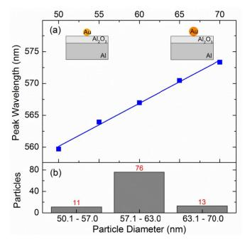
Figure 5. Gold nanoparticle scattering spectra peak wavelength shift as a function of a gold particle diameter for 4 nm and  $16 \text{ nm Al}_2O_3$  thicknesses (a), the particle size-distribution histogram (b).
