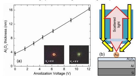
Figure 1. (a) Aluminum oxide thickness as a function of anodization voltage. The insets show dark-field microscopy images of gold nanoparticles at anodization voltages of 0 V and 9 V. (b) Schematic of the measurement and sample geometry.
