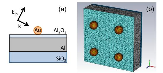
Figure 3. (a) Schematic of the simulated structure and the incident plane wave orientation and polarization, and (b) Numerical simulation model in the software showing the generated tetrahedral mesh with unit cell boundary conditions
