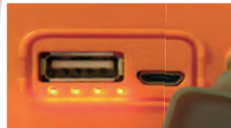
USB for phone charging Micro USB for Lantern charging LEDs showing battery level
