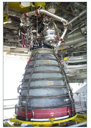
An RS-25 engine sits at the A-1 Test Stand at Stennis Space Center prior to complete installation and testing.
