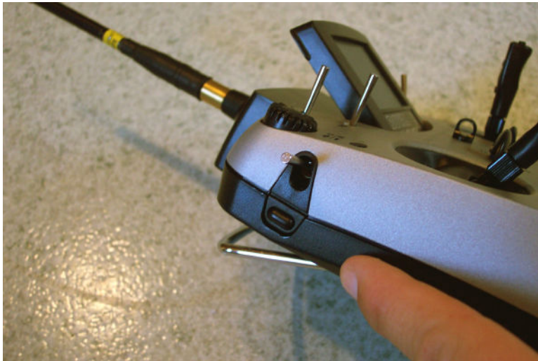
There are two button switches which are located on each side of the transmitter case.
