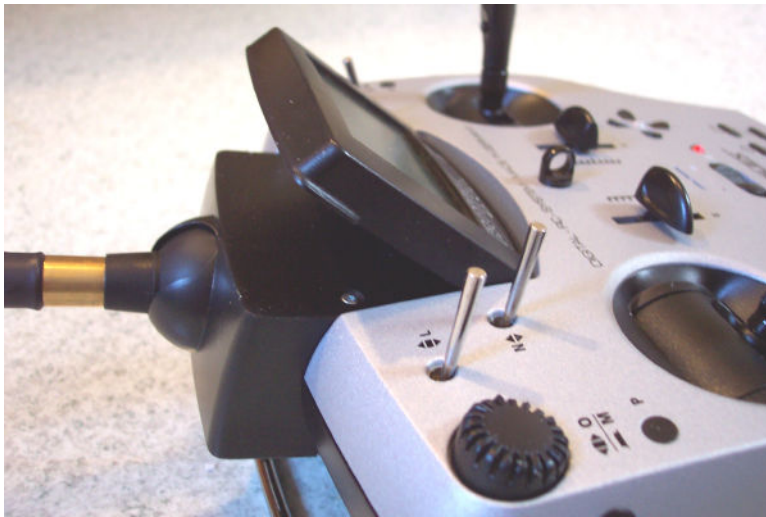
There are two round buttons near the top left and right of the transmitter case. These are called the Digi-Adjusters (DA).
