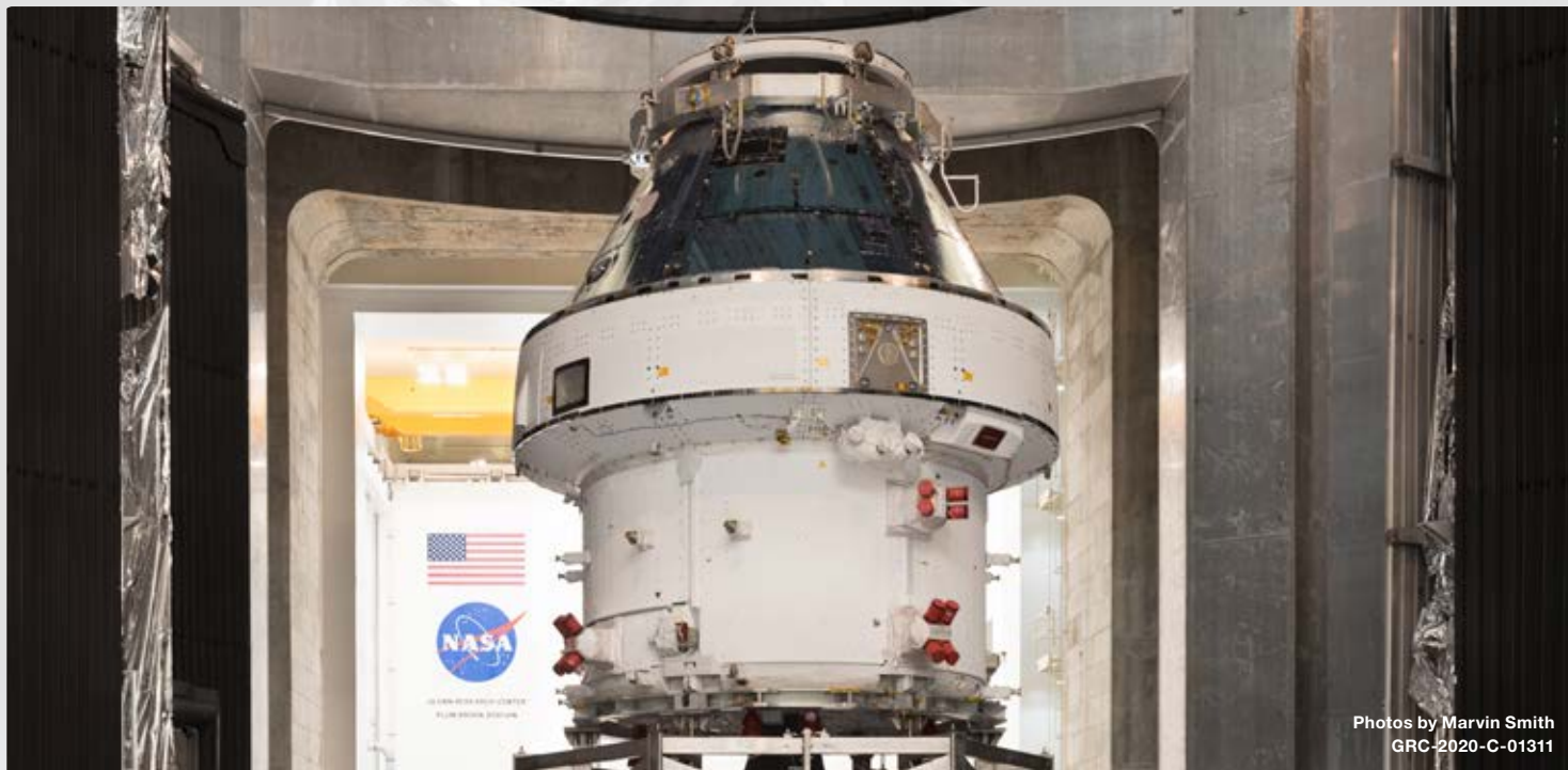
The Orion spacecraft in the Space Environments Complex vacuum chamber.
