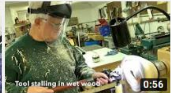
Lubricate the coring groove!
