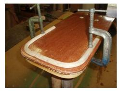
This type of reed molding is often used on original carriages of the brass automotive era as trim. It will be attached using wood working glue and brads. The brad holes will be filled when sight imperfections in the fender surfaces are repaired.
