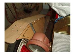
The picture on the right shows one of the completed fender splash shields that will be attached to the fender using a fastener called a "screw rivet", available from:
