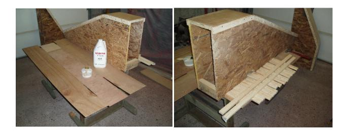
NOTE: Make sure you have everything ready as shown in these two pictures before starting. Notice the grain on the center piece shown in the picture on the left. Observe how it is opposite to the top and bottom piece. Also, the center piece had to be extended by adding a short piece. It will be sandwiched along with its matching piece in the center of the stack. (Increase the magnification on your viewer if necessary)...
