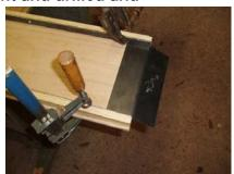
A simple under fender mounting bracket can be made from 1/8" X 2" X 2" angle. Slots on both sides are cut to fit fender irons. A hole at the rear "U" bend will accept a 5/16 X 4" eye bolt to attach fender to fender iron. Measurements for this bracket are up to the builders preferences. Sketches of the bracket on the following page shows the simplicity of it...
