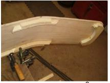
stock material (avoid using plywood). A lap joint is used where ever side pieces are to be joined later.
