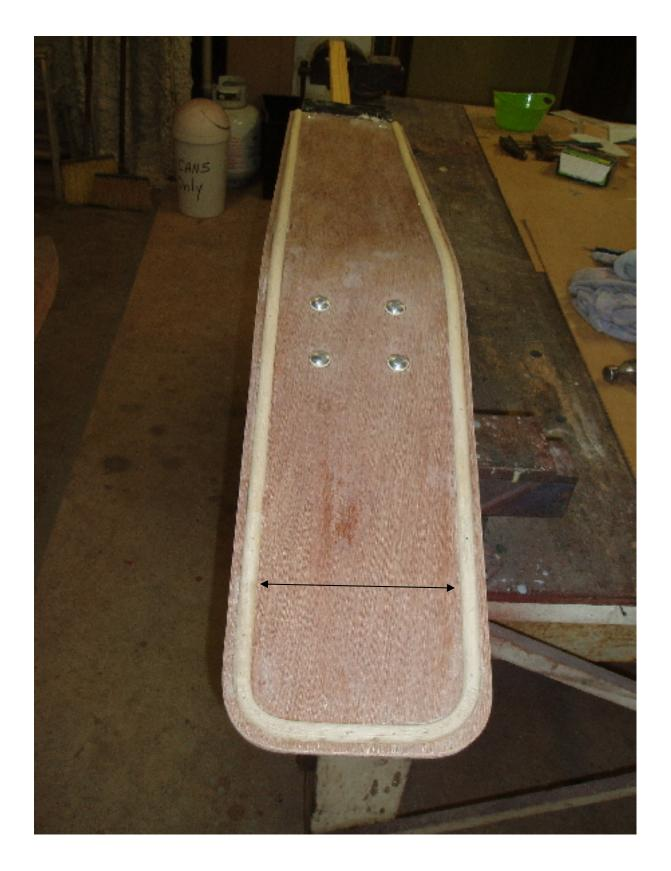
As seen in picture of installed bead on the previous page, a good tight & straight joint is barely visible after installation & can easily be filled for finishing. The correct amount of body filler should be added (using finger) along each side of molding & feathered (sanded) accordingly. This will make the molding resemble one that has been rolled onto the wooden surface...
