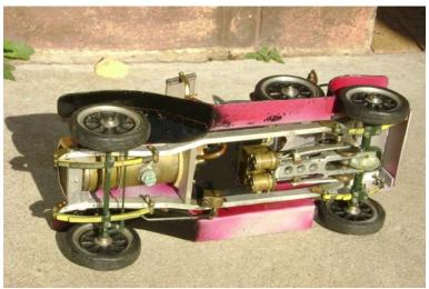
The engine is a twin, double acting and runs on about 10 psi with the steam being generated by the use of Butane gas firing. I have no idea of what scale it ends up as.
