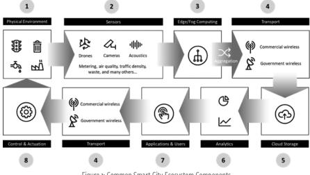
Figure 1: Common Smart City Ecosystem Components
