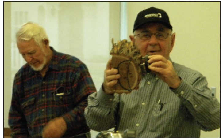
Howard shows how you can use a faceplate as a four-point drive for turning natural edged work pieces.
