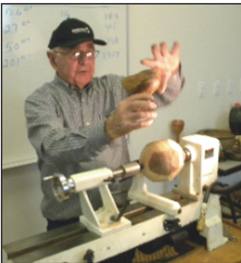
Howard explains the use of a vacuum chuck for hold your workpiece on a lathe.
