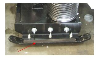
Fig. 17 – Pick-Up Head Skid Spacers.
