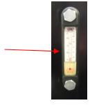
Fig. 31 – Hydraulic Fluid Sight Gauge.
