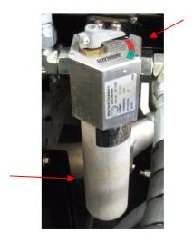
Fig. 29 – Hydraulic Fluid Pressure Filter Housing (Driver side).
