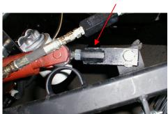
Fig. 11 – Curb Broom Turnbuckle.
