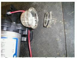
Fig. 26 – Cleaning the Dust Suppression System Water Pump Strainer.
