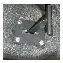
Fig. 5 – Inside view of Cab with T-Handle Control Lever (Non-Broom model).
