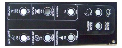
Fig. 8 – Control Panel on Broom model.
