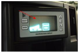
Fig. 6 – Sweeper Power Setting Display – NH Raptor Models
