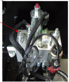
Fig. 13 – Curb Broom Relief Valve.
