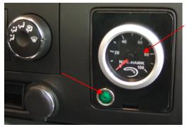
Fig. 7 – Sweeper Power Setting Gauge and Sweep Mode indicator Light – NH 200 Osprey Models
