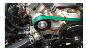
Fig. 23 – Engine Tensioner and Belt - NH 200 Osprey.
