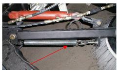
Fig. 12 – Curb Broom Spring.
