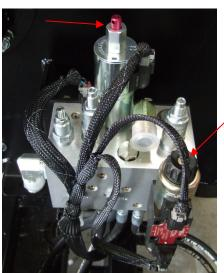
Fig. 9 – Manual Overrides for Hopper (right) and Curb Broom (left).
