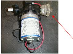
Fig. 25 – Dust Suppression Water System Pump and Strainer (arrow).
