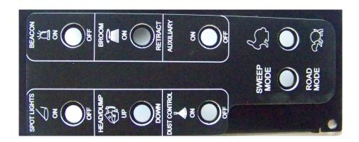
Fig. 4 – Inside view of Diesel Cab Over with Sweeper Control Panel (Broom model).
