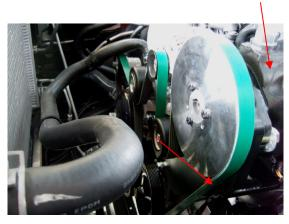
Fig. 22 – Main Hydraulic Pump, Belt – NH 200 Osprey (Driver side).
