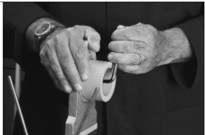
Appliance for manual joining of pipes and fittings by socket welding.
