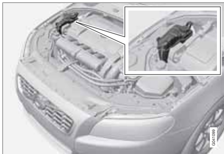
Location of the coolant reservoir
