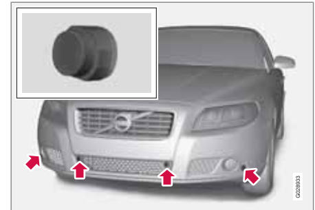
Location of the front sensors
