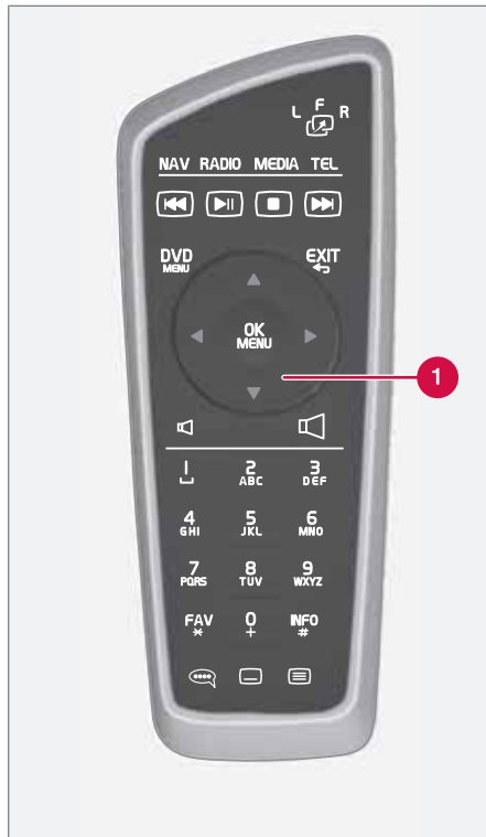
1 The scroll wheel has the same function as TUNE in the center console control panel.
