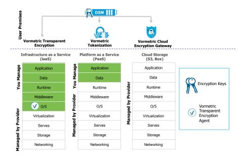
DSM centralizes key management and control of data on-premises, while enabling the protection of data across different cloud environments.
