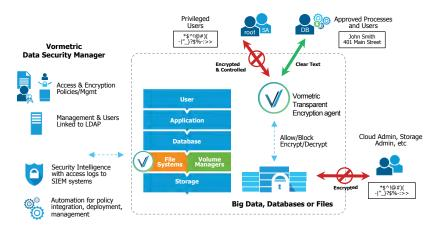
Sample Vormetric Transparent Encryption deployment architecture.
