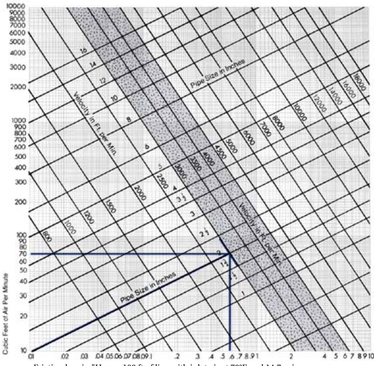
Friction loss in "Hg per 100 ft of line with inlet air at 70°F and 14.7 psia.
