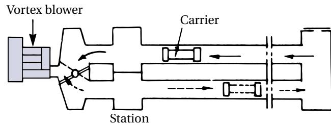
**Pneumatic conveyor.** Vortex vacuum systems convey checks, cash and documents in banks, hospitals, offices, etc. With its reversible operation, the Vortex blower eliminates the need for a diverter valve.
