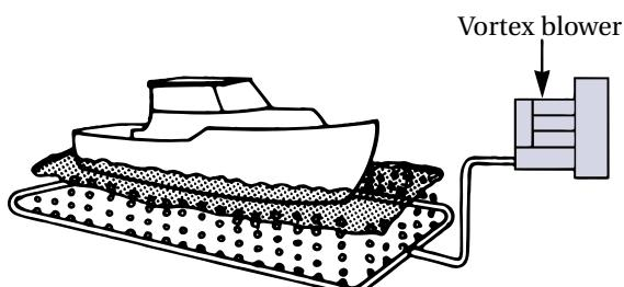
**Ice prevention system.** Air bubbles streaming from a diffuser ring keep water circulating to prevent icing.
