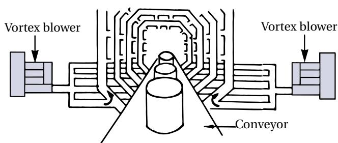
**Component drying.** Air discharge from single or ganged blowers powers a small drying system for parts or products.
