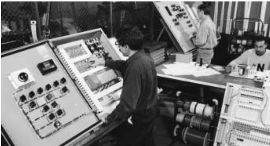
*In-house assembly of control panel with PLC and operator interface terminal.*
