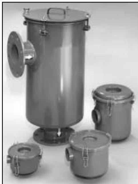
Inline filters have two connections and are typically used in vacuum applications to keep dust and abrasive particles from entering the blower through the connected piping. Filtration efficiency is >99% per SAE Fine Dust Test (10 micron particles). The pleated paper filter elements are replaceable. These filters have a low pressure drop and use a positive sealing O-ring system.
