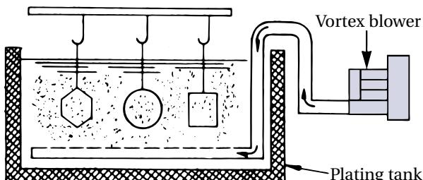
**Plating tank agitation.** High-pressure air circulates the electrolytic solution in a plating bath to promote uniform, rapid plating.
