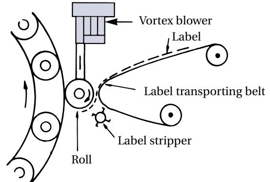
**Automatic labeling machine.** As a label stripper frees labels from their backing paper, they are held by suction on a roller for transfer to labeling equipment.
