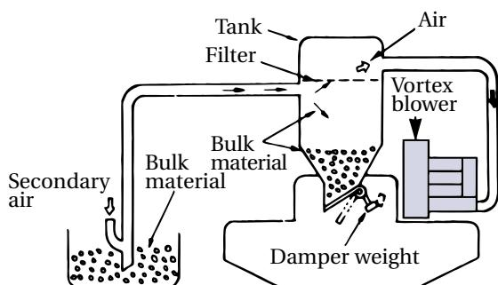
**Bulk material handling.** Air transport systems use Vortex blowers to convey dry materials such as pellets, granules and chips with either vacuum or pressure.
