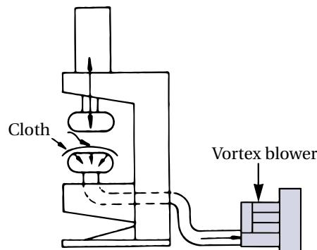
**Commercial ironing machine.** In this ironing machine, clothing is ironed on a padded surface with the aid of steam. The Vortex blower sucks the steam through the padded surface for evacuation.
