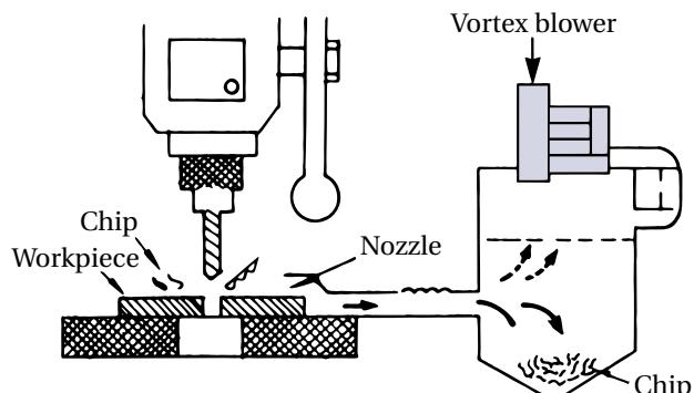
**Chip removal.** Chips generated during operations are automatically evacuated by a Vortex vacuum system.
