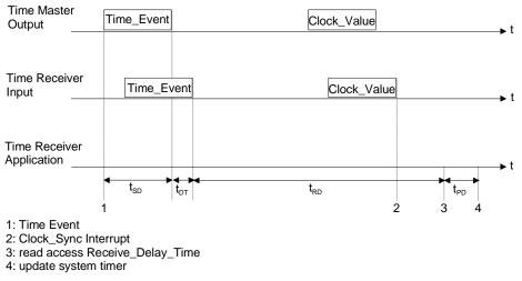
Figure 7-20: clock synchronization mechanism
