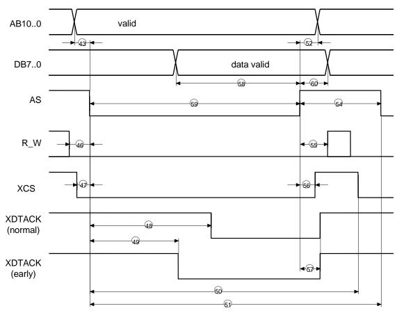
Figure 10-19: Asynchronous Motorola Mode (WRITE)
