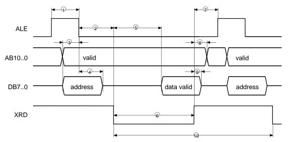
Figure 10-9: Synchronous Intel Mode, READ (XWR = 1)
