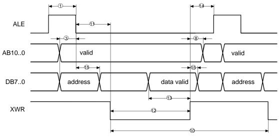
Figure 10-10: Synchronous Intel Mode, WRITE (XRD = 1)
