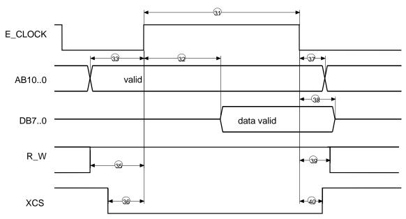
Figure 10-15: Synchronous Motorola-Mode, READ (AS = 1)
