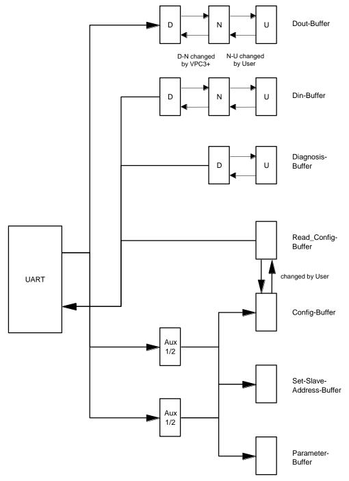
Figure 6-1: DP\_SAP Buffer Structure
