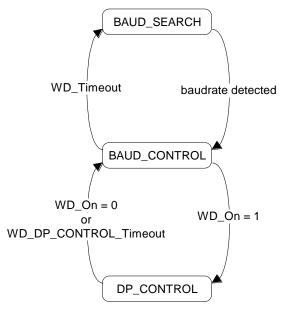
Figure 5-12: Watchdog State Machine (WD\_SM)
