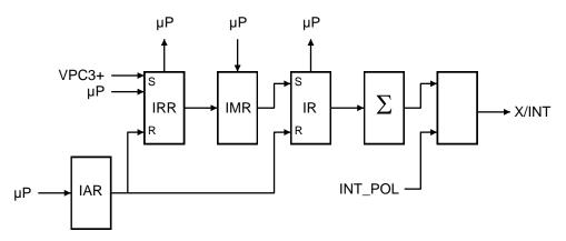
Figure 5-8: Block Diagram of Interrupt Controller
