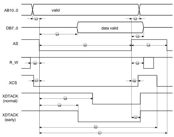
Figure 10-18: Asynchronous Motorola Mode, READ (E\_CLOCK = 0)
