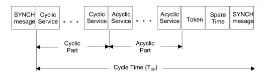
Figure 7-15: Telegram sequences in IsoM with one DP-Master (Class 1)
