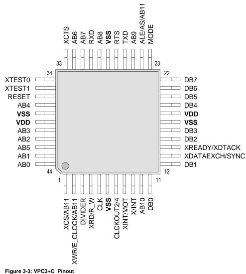
Figure 3-3: VPC3+C Pinout
