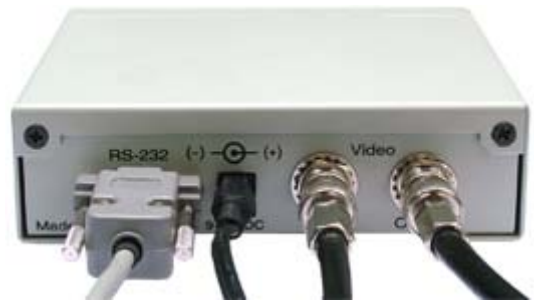
Figure 211: VSIB Connection Cables
