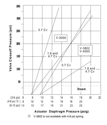
Figure 11: Closeoff Pressures 2-Way Normally Open or 3-Way Normally Open Port Valve with V-3000-1 (31), V-3000-2 (32), V-3802-1 (39), or V-4000-1 (41) Pneumatic Actuator
