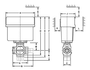
Figure 7: VT Series Valve with Electric Actuator (20, 22, 50, 51 or 52) ①
