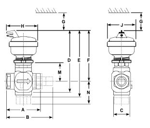
Figure 4: VT Series Valve with V-4000-1 (41) Pneumatic Actuator ①
