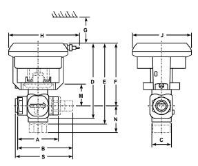
Figure 5: VT Series Valve with V-3000-1 (31) or V-3000-2 (32) Pneumatic Actuator ①
