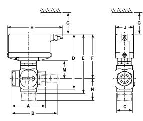
Figure 6: VT Series Valve with V-3802-1 (39) Pneumatic Actuator ①
