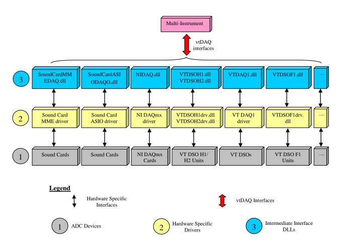
The following diagram shows how Multi-Instrument communicates with different types of DAC hardware via the standard vtDAO interfaces.
