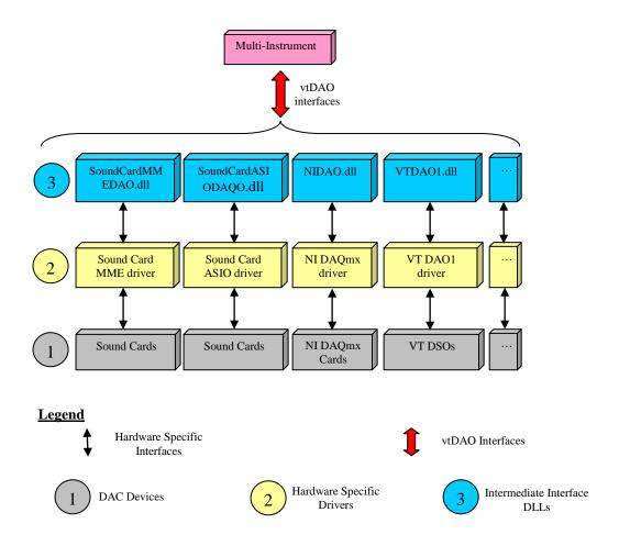
You can write your own back-end program to interface to the ADC and DAC devices that are supported by Multi-Instrument via vtDAQ and vtDAO interfaces. As all these devices conform to the same interface standard, you only need to write the interface codes in your program once and your program will support all these devices.
