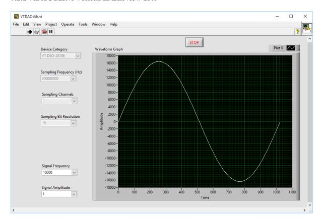
vtDAOdds.vi is a sample VI for Labview programming using vtDAO interfaces. VtDAO interface wrapper: vtDAOLV.dll, is called using Labview Call Library function node. It is basically a signal generator VI with adjustable sampling parameters, signal frequency and signal amplitude. To keep the VI simple, these parameters cannot be changed on-the-fly.
