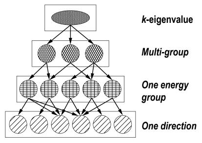
*Example: neutron transport in reactor*
