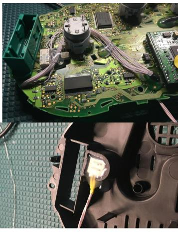
Use a rotary tool to trim an opening in the white plastic shroud to fit the ColorMFA screen. It is necessary
