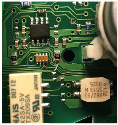
Immo 2 Lowline and Midline clusters only have 6 warning light provisions instead of 8. The LED's are also turned 90\*. As like Immo 3, they need removed and jumpered with the supplied SMD resistors then Trinput wires soldered according to the diagram below.
