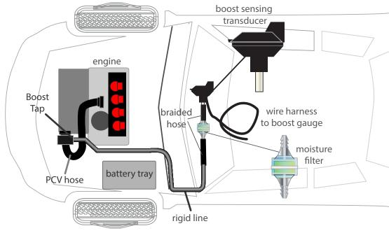
Inside the cabin, the plastic vacuum line from the engine is connected to the vacuum/boost transducer. A moisture filter is installed between the vacuum source and transducer. The transducer wiring harness is routed to the gauge later.
