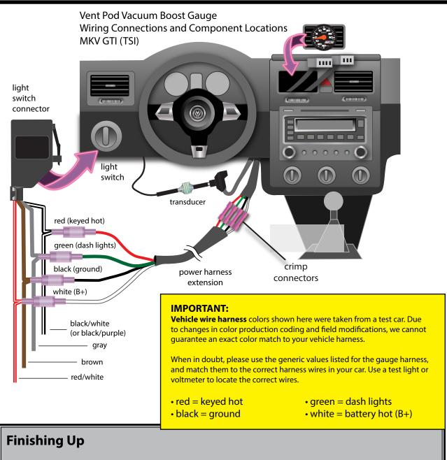
Splice the power and headlight harnesses using the bullet connectors in the kit.
