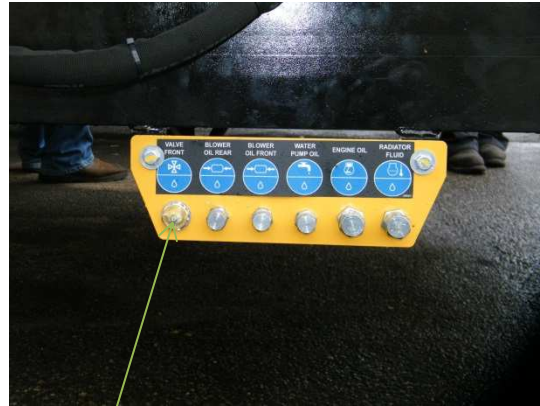
4-WAY VALVE GREASE POINT
