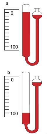
Figure 2.03. An ideal gas thermometer.
