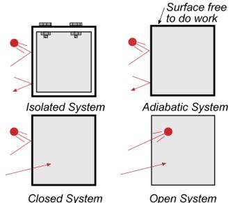
Figure 2.01. Systems in relationship to their surroundings. The ball represents mass exchange, the arrow represents energy exchange.
