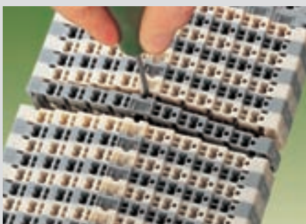
Open the assembly by laterally sliding a block using a screwdriver (2.5 x 0.4) mm . . .
