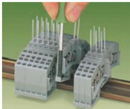
Detaching: separate terminal strip, displace individual terminal block laterally and remove from the carrier rail
