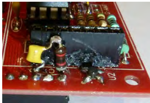
Figure 4, adding 82R in series to C7.
