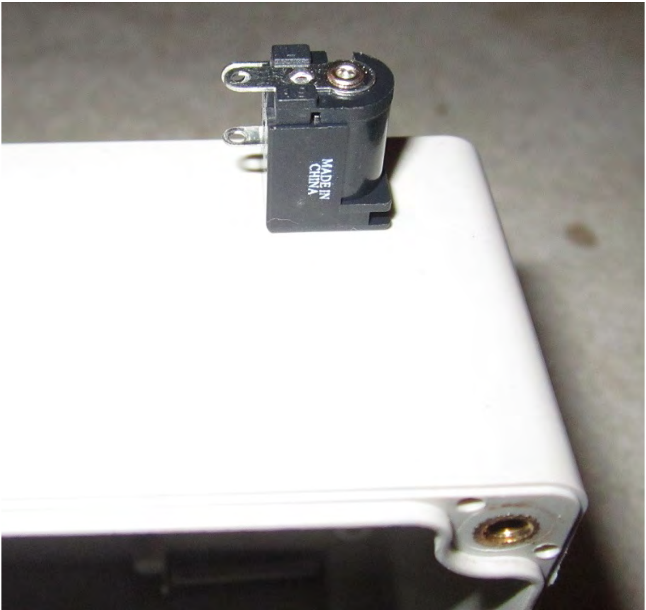
Figure 25. Figuring out where to drill hole for wall wart connection.
