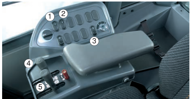
1:Cut-off ON/OFF switch 2:Cut off adjustment switch 3:Fan reverse ON/OFF switch 4:Boom control 5:Bucket control
