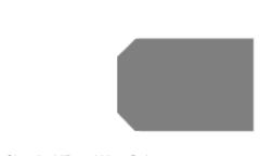
In certain applications that require the use of ultra-hard and brittle substrates of Silicon Carbide, Sapphire, or GaN materials, such as those associated with the manufacture of Light Emitting Diodes (LEDs), a different type of edge treatment is sometimes deemed appropriate. This type of edge treatment is often called a "Bevel Nose."
