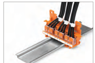
Vertical mounting with strain relief plate on DIN 35 rail. Wiring locations identified by marker strips (210-334)
