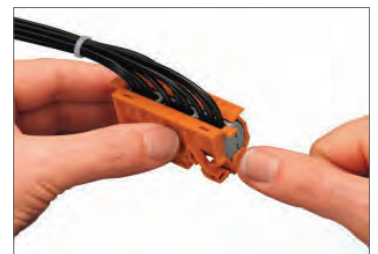
222: Inserting or removing connector from the end of the carrier, securing with snap lock
