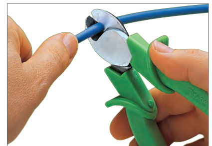
Cutting of cable
