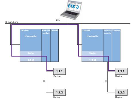
In this application example, the WAGO KNXnet/IP controller with the KNX/EIB/TP1 module is used as a router on an IP backbone (Ethernet). No IEC application is required for the router functionality. The ETS 3 is connected on the Ethernet side and has access to all devices, which are connected via the KNX/EIB/TP1 modules in the TP1 networks shown. A device in the TP1 network on the left can communicate with a device in a TP1 network on the right via the IP backbone.
