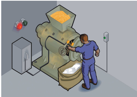
Fig. 6: Safeguarding a grinding mill with guard door lock in Task 1
